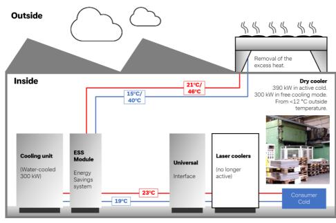
Installation of a central cooling system (Plug&Play). 300 kW at 19 °C process water temperature including an energy-saving circuit and passive cooling from an outside temperature of 12 °C.
