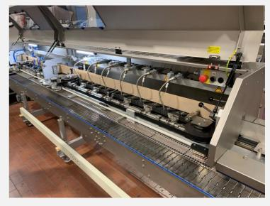
In the first belt station, the splice is heated to softening temperature using heating elements. To prevent the sensitive outer surface of the bag from sticking to the hot parts and being damaged, a teflon-coated steel belt runs along. The glued surfaces are then pressed together with grooved pressure rollers (crimp rollers) and cooled to below the softening temperature of the adhesive in the second belt station.
